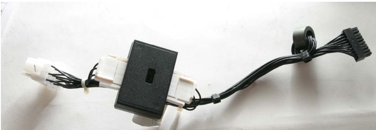
Figure 4: The completed harness with the flash controller attached is shown above.
