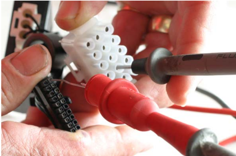
Figure 3: Probes are shown positioned for ohming out the pin 11 wiring on Molex and micro amp plugs.
